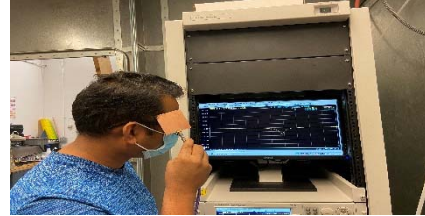
Fig. 14. S_{11} measurement setup brought close to a human head.
