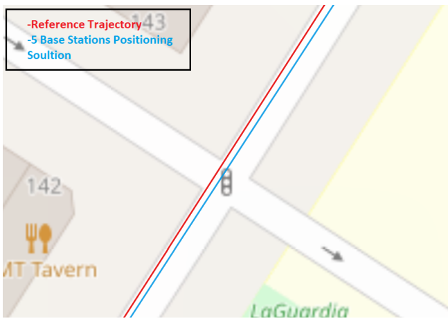
Fig. 7. Window of the estimated positioning solution (5BSs scenario) versus the reference trajectory
