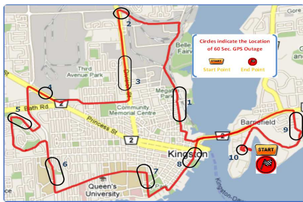
Fig. 10. Road Test Trajectory and circles indicate the approximate locations of 60-second GPS outages.
