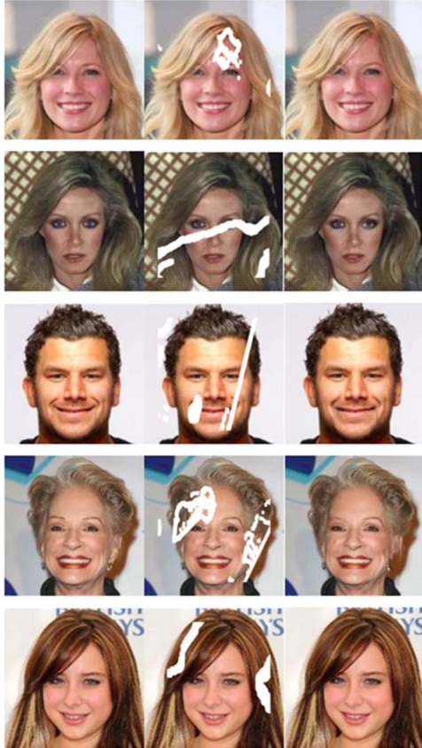
Fig. 2. Results from the trained model. Ground truth image on the left, masked image on the middle and recovered image on the right. During testing, only the masked image is used as an input to produce the recovered inpainted image.
